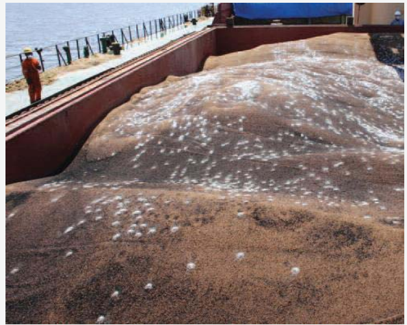
Heat damaged cargo with remaining tablet/pellet residues (blackening)
