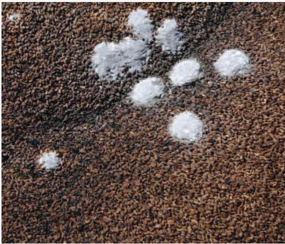
Heat damaged cargo with remaining tablet/pellet residues (blackening)
